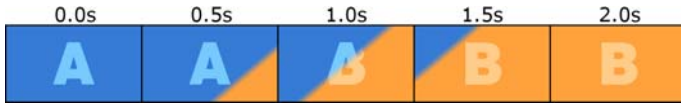
Diagram: Five snapshots from the life of a 2-second diagonal wipe transition.
